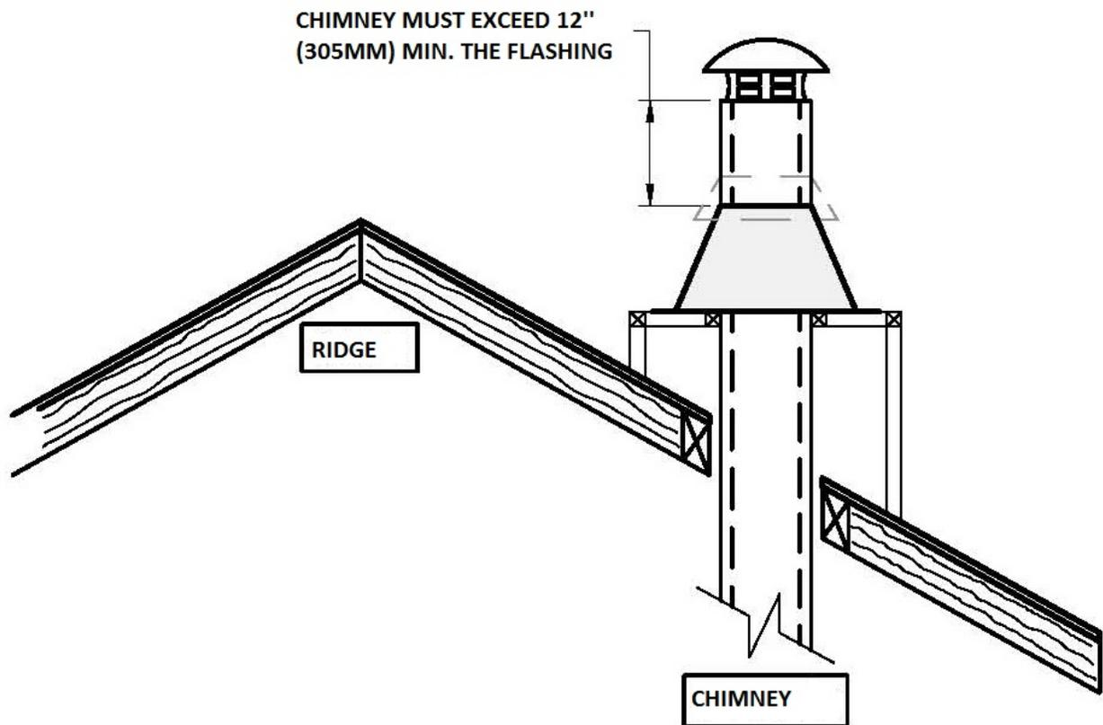
**Note: The chimney chase on the roof must be the same size as the flashing.**
