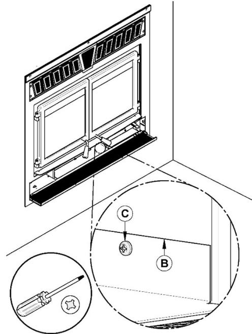
3. Remove and keep the heat shield (B) and the screws (C). 4. Cut the Tie wrap (D).
