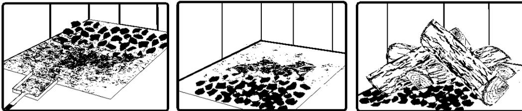
*Remove ash first, and then rake charcoal towards the front of the firebox before loading so that it will ignite the new load.*
