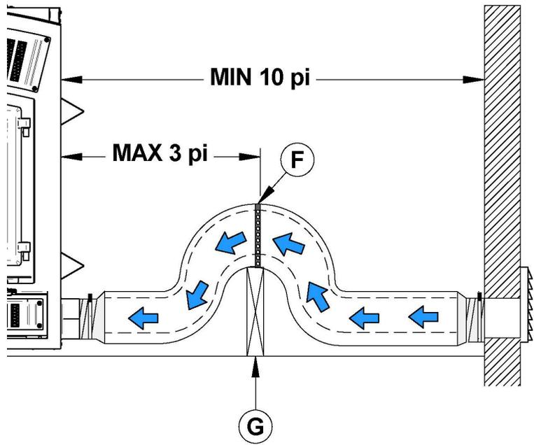
To complete the installation, make a hole of 1/4" to 1/2" (6 mm à 13 mm) bigger than the insulate pipe diameter in the outside wall of the house at the chosen location. From outside, place the outside wall termination in the hole (open side down) and fasten the register to the wall, with screws.
