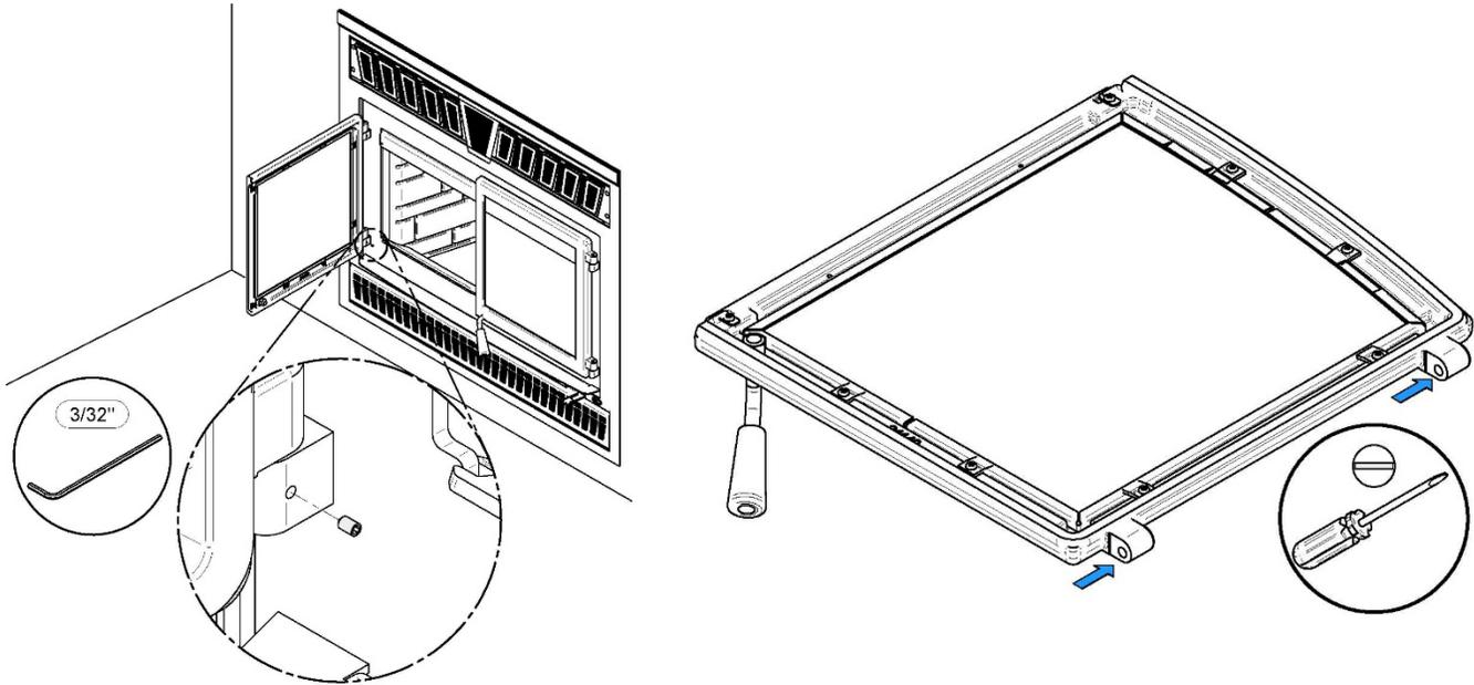
Using a flat screwdriver, turn the adjustable hinge rods in the direction shown to adjust the doors. Tighten all door hinge pressure screws when they are at the desired positions.
