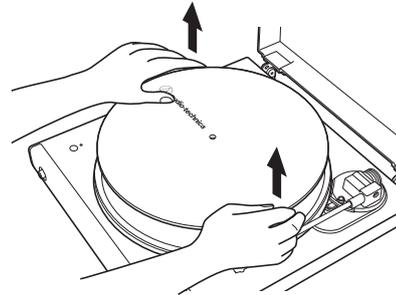
2. Remove the platter, turn the platter over, and then remove the old belt.
