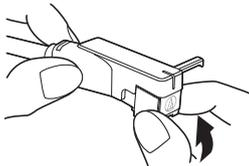
3. Make sure there is no gap between the headshell and the cartridge.
