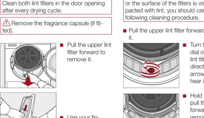
Cleaning the lint filters and air flow openings thoroughly If the drying duration has become longer
