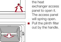
A guide pin in the dryer will come out which prevents the access panel from closing without the plinth filter.
