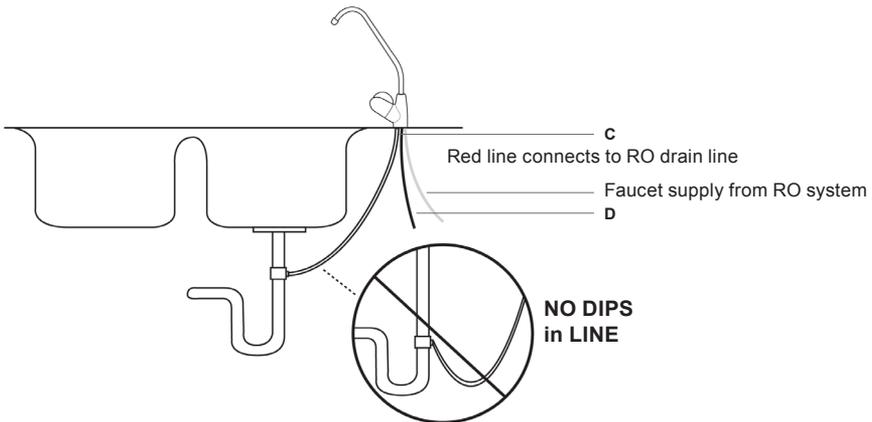
as possible and that there are no dips, loops, low spots or kinks. (See D in Figure 2 above). Also, to reduce noise, assure that RO drain line enters the vertical pipe from a direction other than the direction of entry of the garbage disposal pipe.
