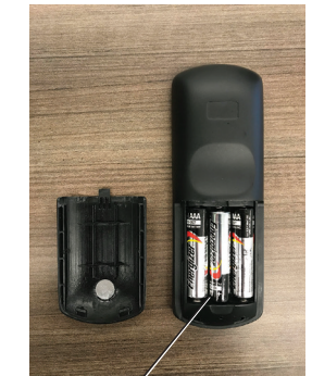
Insert (3) AAA Alkaline Batteries
