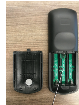
Polarity Markings Inside the Battery Compartment
