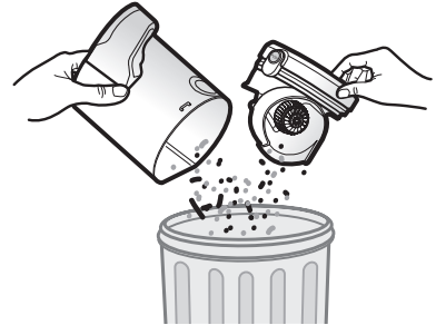
3 Remove dust in the dustbin and cyclone unit
