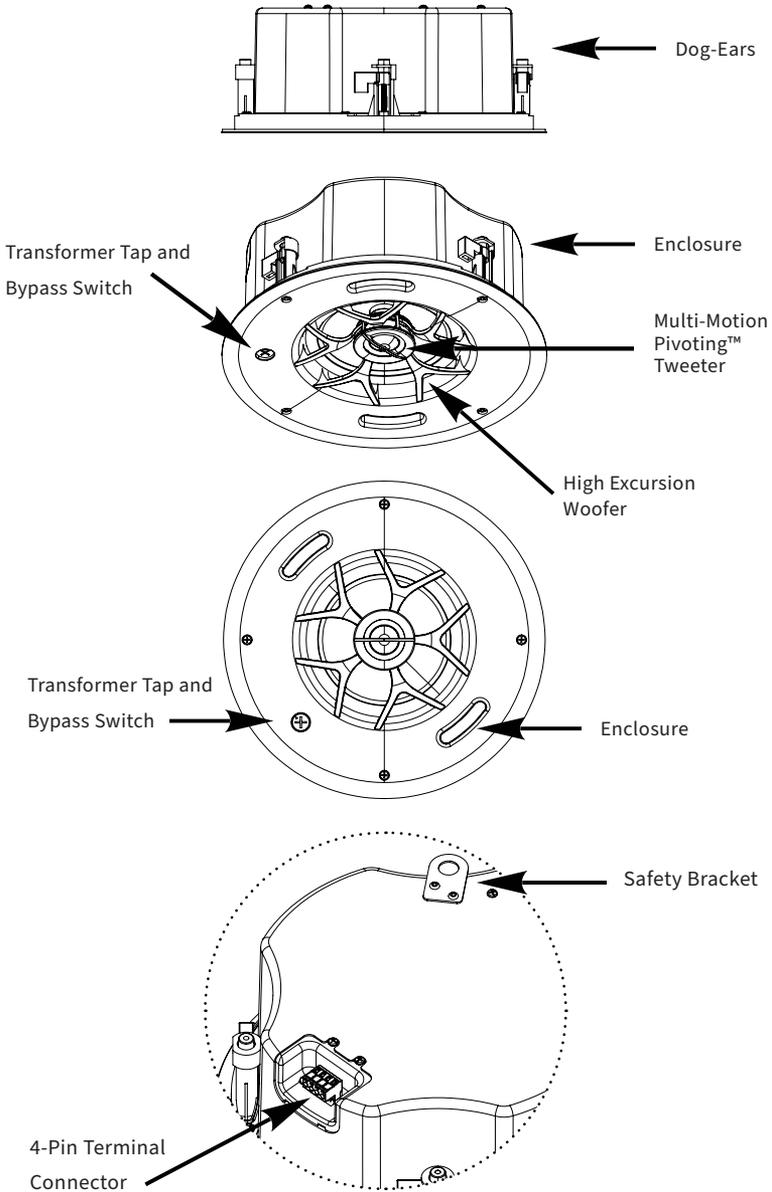
**CUT OUT DIAMETER** 10 1/2" (266mm) | **MOUNTING DEPTH** 4 23/64" (110mm)
