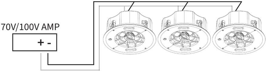
Wiring Diagram for 6Ω system
