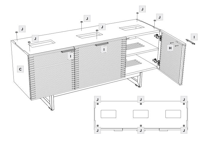
Place (K) Glass Top on top of (C) Cabinet. Position glass flush with cabinet front doors.
