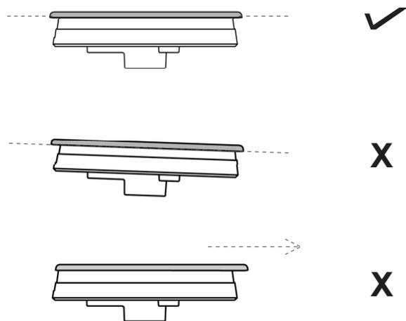
The burner grates must be properly placed inside the recess on the cooktop.
