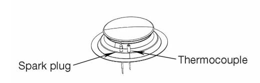
Push and turn the knob to the maximum gas position to induce a flame into the desired burner.
