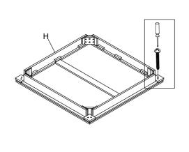
STEP: 2 Place the table top (H) upside down on a soft and flat surface. Assemble table leg (I) by using Allen Key (7) with hardware 2, 5, and 6.
