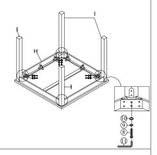
STEP: 3 To level the table, stand the table up on a flat surface and tighten all the bolts by using Allen Key (7).
