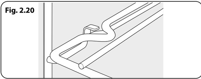
Any shelf can be fitted in any of the positions. The oven shelves are retained when pulled forward but can be easily removed and refitted.
