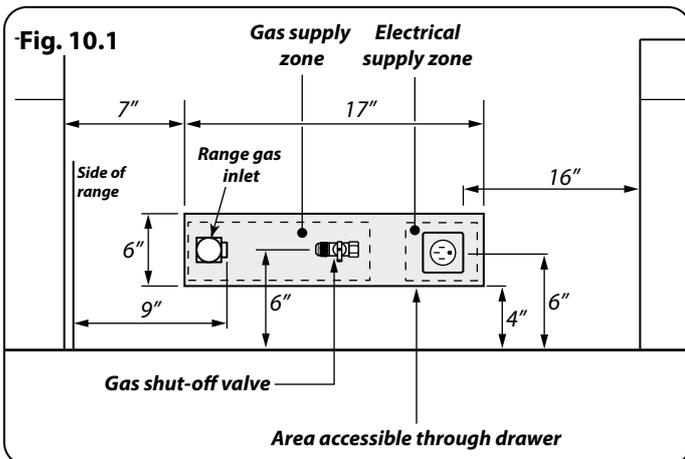
Installation of this range must conform with local codes or, in the absence of local codes, with the National Fuel Gas Code, ANSI Z223.1-latest edition.
