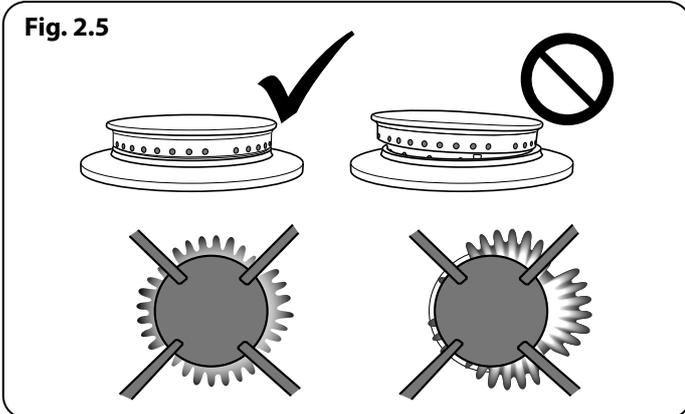
If the flame is distorted, check that the burner head is correctly placed over the burner base (**Fig. 2.5**)
