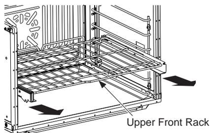
If extension racks are difficult to extend, lubricate the racks with the graphite lubricant provided with your oven. Remove the rack from the oven, remove debris in the slide tracks with a paper towel, shake the graphite lubricant and place 4 small drops on the two bottom tracks of the left and right sides. Open and close the rack several times to distribute the lubricant.
