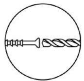
Match the drill bit to the wall anchor and hole size.
