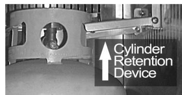
Type 1 20lb cylinder with an over-fill protection device.
