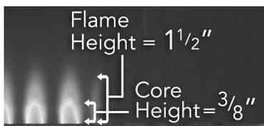
The flames should burn quietly (no "torch" sounds) and they should not "lift" up from the burner.
