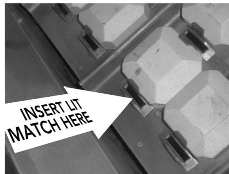
The ProSear™ burner does not feature a manual lighting tube.
