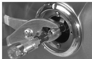
The proper setting is where the flame is stable at its lowest setting. A slight flutter will be present in the crossover portion of the front of the burner before the burner itself becomes weak.
