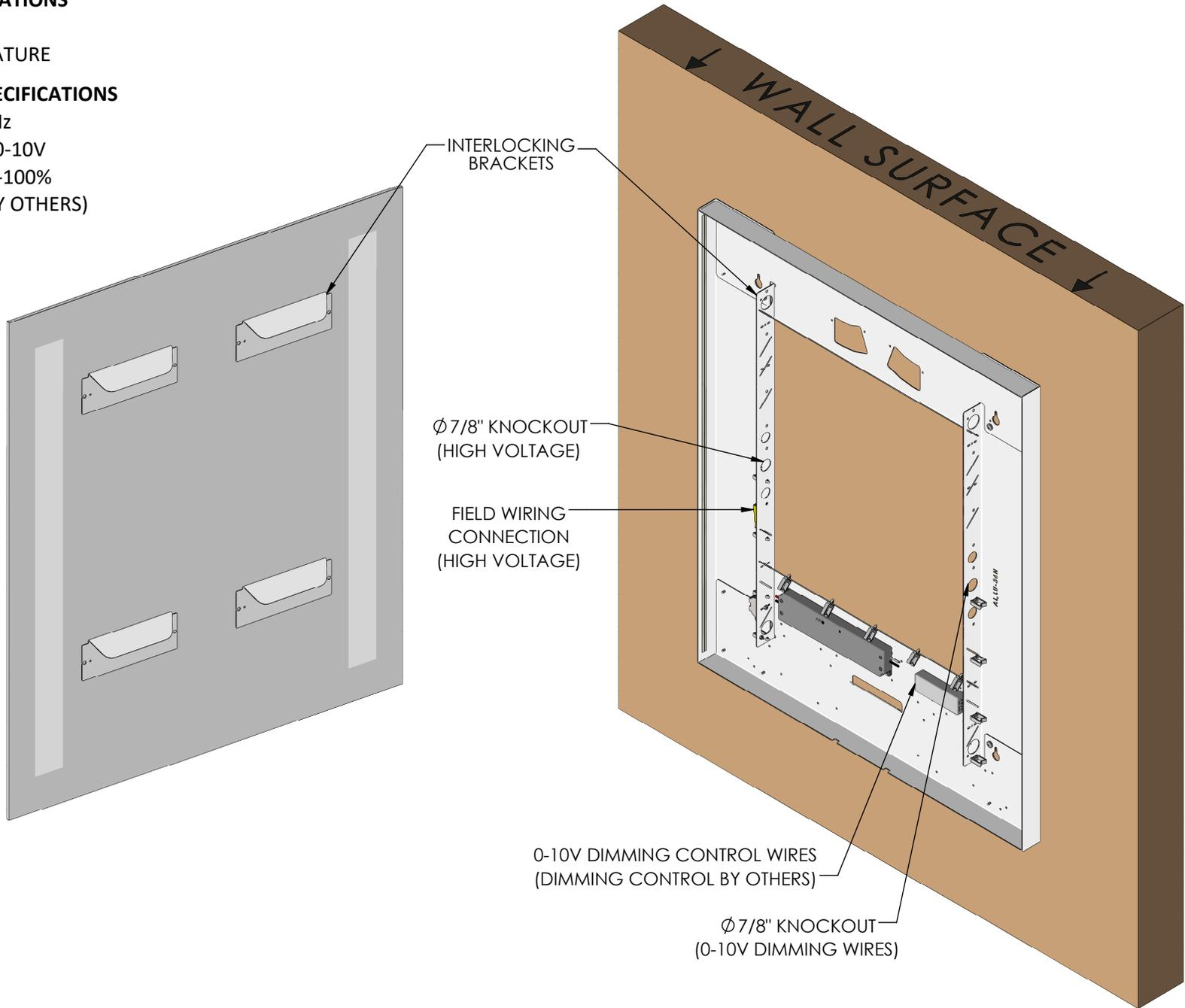
0-10V DIMMING CONTROL WIRES
