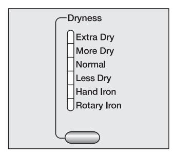
■ Press the selection button until the desired indicator illuminates.
