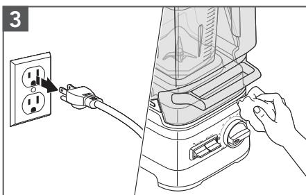
Unplug before cleaning. Wipe the base and the cord with a warm, damp cloth and dry with a soft cloth.
