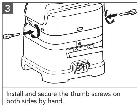
Install and secure the thumb screws on both sides by hand.
