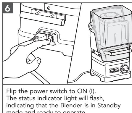
Flip the power switch to ON (I). The status indicator light will flash, indicating that the Blender is in Standby mode and ready to operate.
