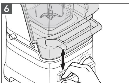
When finished, flip the START/STOP toggle switch up or down to stop.
