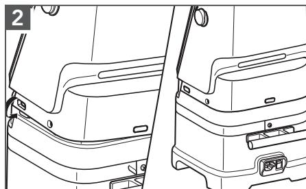
Secure both sides over the tabs on the either side of the blender base.
