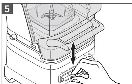
Using the Pulse mode (optional): Press and hold the PULSE toggle switch up for a faster pulse, or down for a slower pulse.
