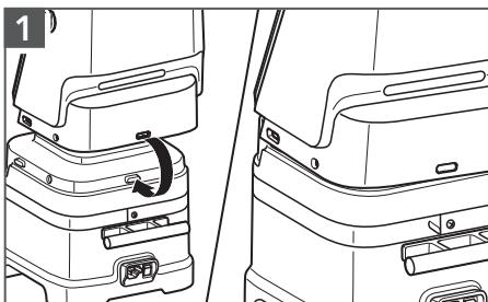
Install the back cover by aligning the tab on the rear side of the base with the slot on the back cover.
