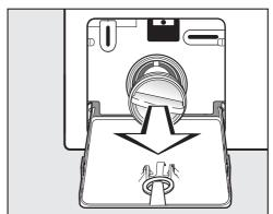
■ Remove the drain filter completely.
