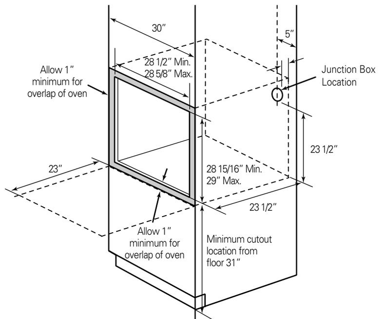
**2 INSTALLATION DRAWINGS (FOR 30" DOUBLE BUILT- IN OVEN)**
