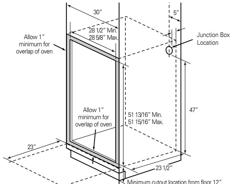
**3 INSTALLATION DRAWINGS (FOR 30" SINGLE BUILT-IN OVEN UNDERCOUNTER)**
