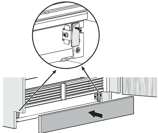
Remove the backing foil and affix the toe kick panel.
