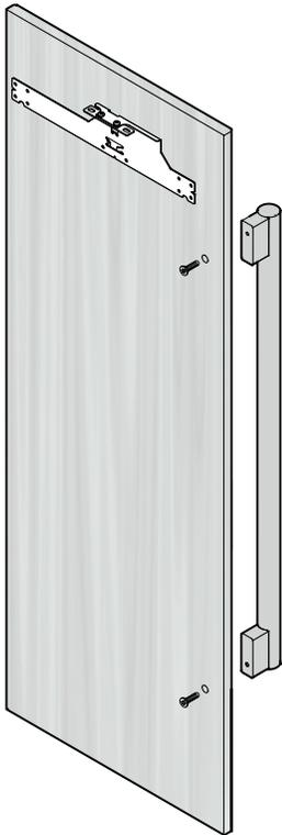
Only use countersunk screws for handle mounting.
