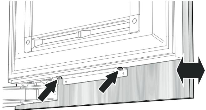
Fasten the panel through the bottom attachment bracket with two screws 4 x 14.
