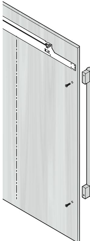
Only use countersunk screws for handle mounting.
