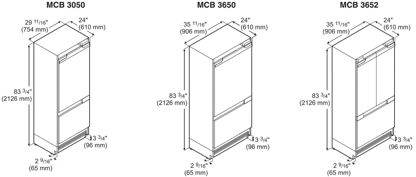
Stated minimum height dimensions include when the levelled feet are fully inserted.
