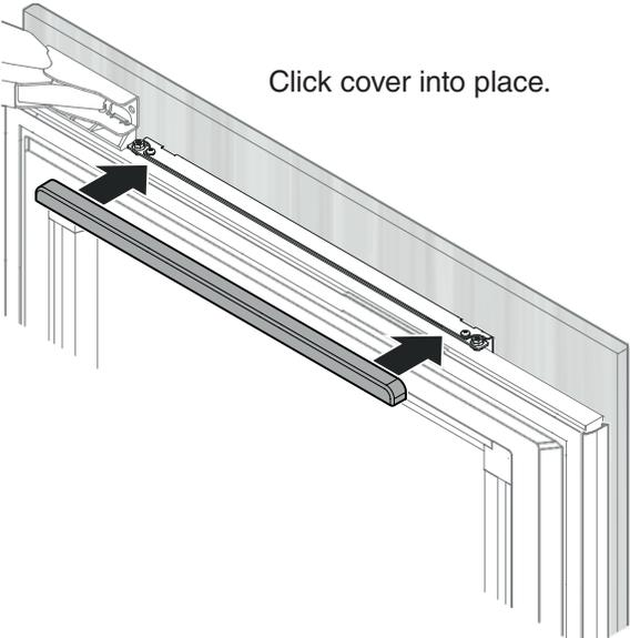
Hook the door cover strips at the front of the supports and snap in at the back.
