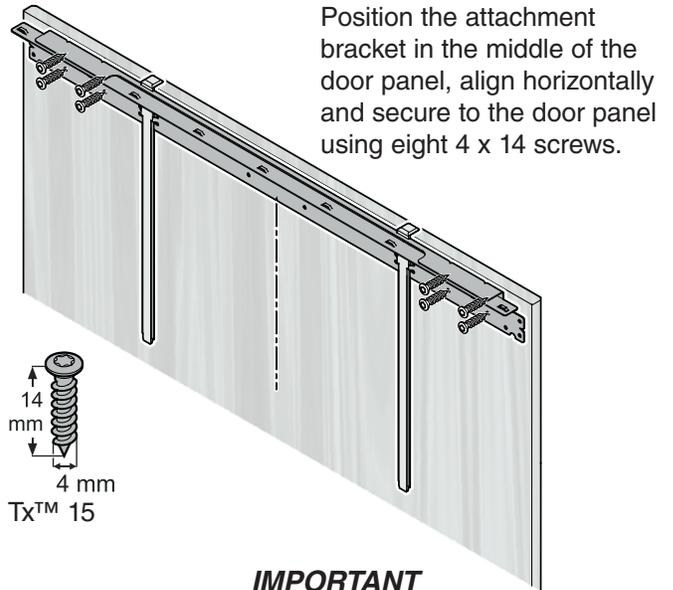
Position the attachment bracket in the middle of the door panel, align horizontally and secure to the door panel using eight 4 x 14 screws.
