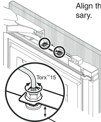
Loosen the hex nuts and turn the adjusting bolts with the Torx 15 key provided.
