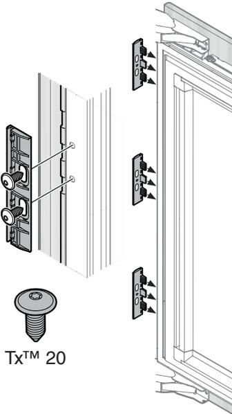
Fasten the panel through the bottom attachment bracket with two screws 4 x 14.
