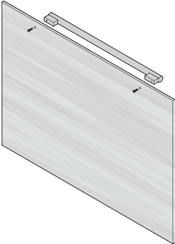
Only use countersunk screws for handle mounting.
