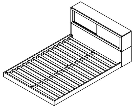
DO NOT TIGHTEN BOLTS UNTIL COMPLETELY ASSEMBLED /
