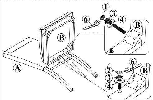
Step 1: Place the Chair Back (A) on the floor. Attach Seat Box w/Seat Cushion (B) to the Chair Back (A) by inserting the Short Bolt (2), Lock Washer (3), Flat Washer (4) into the holes at the rear bar of the seat frame. Attach Long Bolt (1), Lock Washer (3), Flat Washer (4) into the holes at the rear corner block of the seat box. Tighten all Bolts with Wrench (6). Do not fully tighten.
