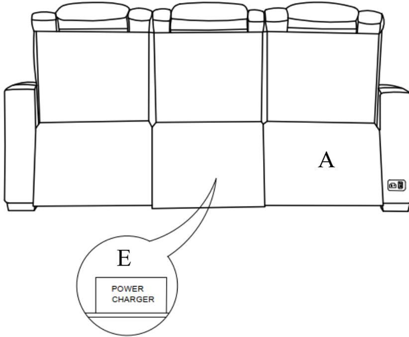
Step 4: Connect the Power Cable 29V (E) to the power socket on the back of Seat (A).
