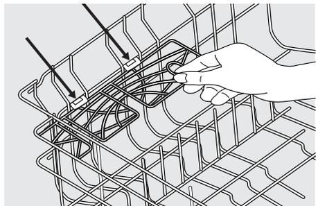
Place the clips of the cup shelf over the horizontal rack wires and push down to attach the cup shelf onto the second wire of the upper rack.
