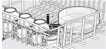
Some models have fold-down cup shelf or a cup shelf/stemware holder. They can be used to load two levels of cups, juice glasses, and other short items. Stagger items on upper level so that water can reach all inside surfaces. Fold up to load tall glasses.
