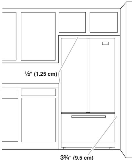
To ensure proper ventilation for your refrigerator, allow for a 1/2" (1.25 cm) space on each side and at the top. Allow for 1" (2.54 cm) of space behind the refrigerator. If your refrigerator has an ice maker, make sure you leave some extra space at the back for the water line connections.
