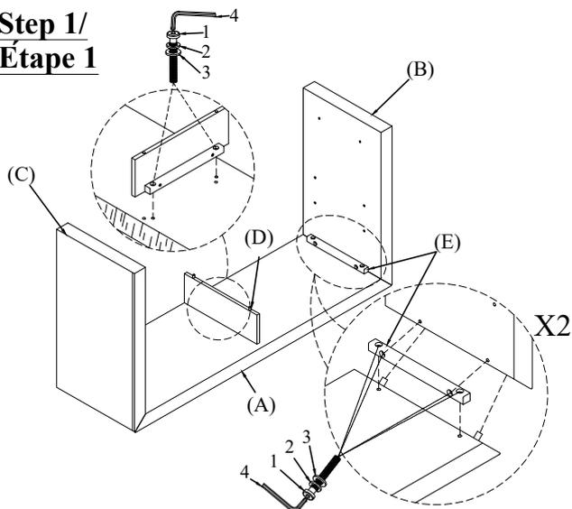
DO NOT TIGHTEN BOLTS UNTIL COMPLETELY ASSEMBLED.
