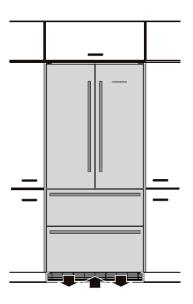
CS 20 appliances don't need any ventilation openings in the cabinet. The required airflow is directed through the toe kick area.
