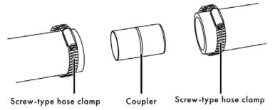
Secure the drain hose to the air gap, waste tee, or garbage disposal with a screw-type clamp, using the appropriate method below. See "Drain Preparation" on page 9 if you do not know which method to use.
