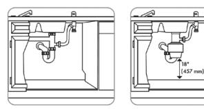
Method 2 - High drain with a waste tee or garbage disposal connection
