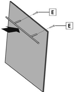
3. Put the hook into the slot of the outer door for the positioning.
