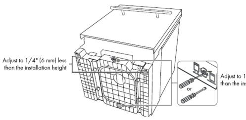
Adjust to 1/4" (6 mm) less than the installation height
