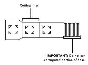
If a longer drain hose is required, you can add up to 42" (1067 mm) of length, for a total of 10' (3048 mm) to the factory installed hose. Use 5/8" (16 mm) or 7/8" (22 mm) inside diameter hose and a coupler to connect the two hose ends. Secure the connection with screw-type hose clamps.
