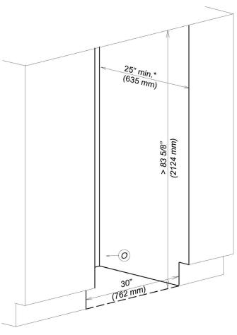
UNIT ACCEPTS A CUSTOM FRONT PANEL (min. 3/4" thick) 83 1/2" - 85 3/16" (2121 mm - 2165 mm) (E) 10 1/4" (260 mm) (W) 2" - 8 3/8" 1 mm - 213 mm) 1 1/8" (29 mm)4 1/8" (105 mm) '168 mm - 216 mm)
