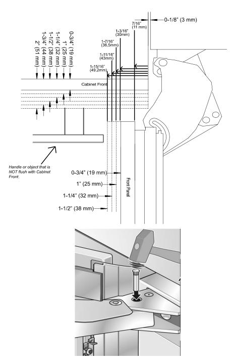
When installing hinge side next to an appliance or object that is within range of the door panel, limit the door opening angle to 90°. This is done by installing the banking pin as illustrated. Insert the banking pin through the holes and drive in with a hammer.
