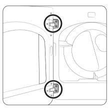
**12.** Reinstall the door on the front frame, and then carefully insert and tighten the 4 hinge screws.
