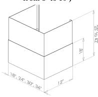
\*Please note that measurements provided reflect the bottom of the hood being 30" above the stove.
