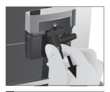
► Remove the milk system from the dual spout.
