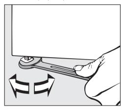
■ The machine can be leveled by turning the legs clockwise or counterclockwise as necessary.
