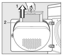
■ Open the door and remove the lint filter, 1, by gently lifting it upwards.
