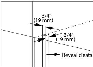
For flush installation you need to two reveal cleats fixed like above figure.
