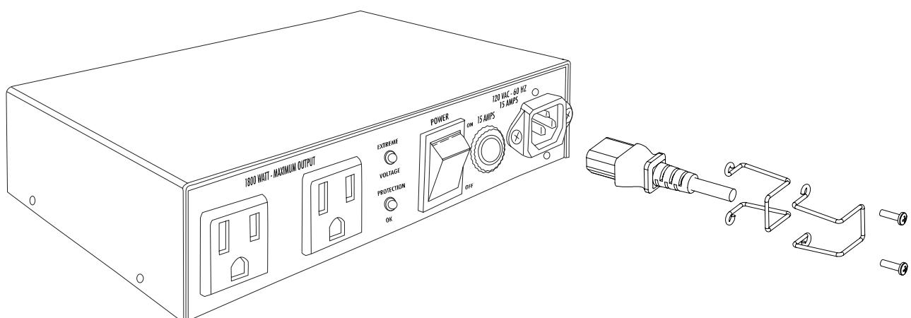
To attach or detach the AC power cord security clamp, simply assemble or disassemble as shown in the above illustration. Place clamp together as shown, and secure screws in the provided holes to lock the power cord in place. Loosen screws and remove clamp from unit to detach.
