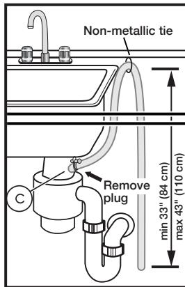
Note: Plumbing installations will vary - refer to local codes. Drain hose included is 90 1/2" (230 cm) and can be extended to a maximum of 168 1/2" (428 cm).
