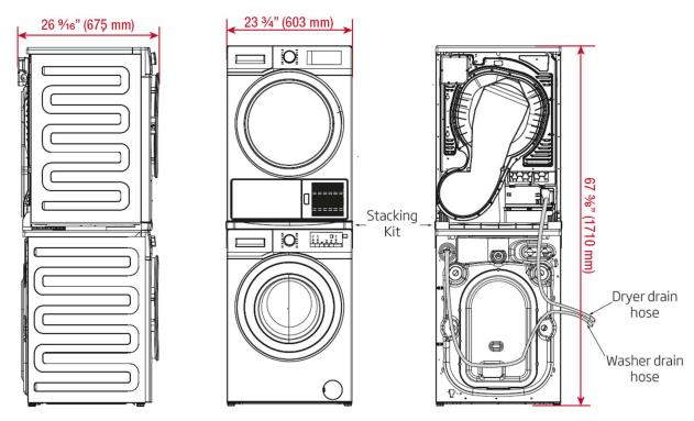
Stacked installation minimum air gap clearances: 6 1/4" top, 1/2" sides, 1/2" back, front 1/2"
