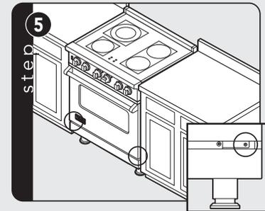
If the door needs to be adjusted, loosen hinge trim screws (see step 2). Adjust the screws located between the door and kickplate using a 5/32" hex head allen wrench. After adjustment, tighten hinge trim screws.
