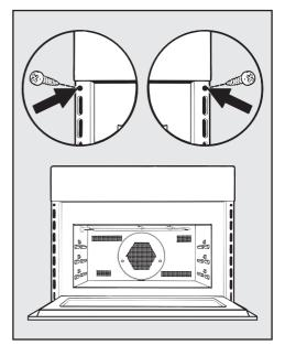
Open the door and use the screws supplied to secure the oven to the side walls of the cabinetry through the holes in the oven trim. Miele uses software to operate and control the appliance.
