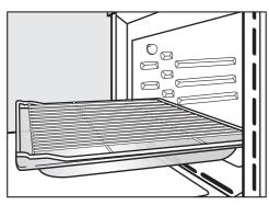
We recommend using the rack together with the glass tray when cooking items on the rack which might drip. **Roast Probe**
