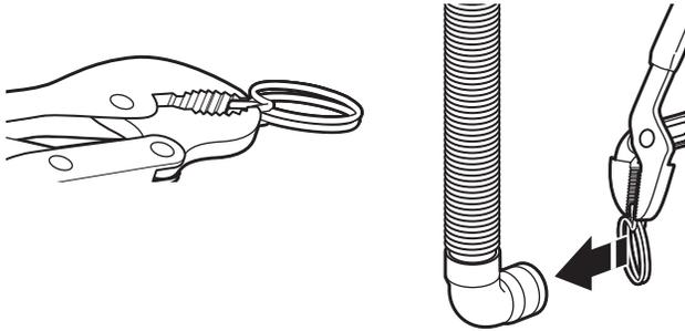
3. Squeeze clamp with pliers and slide elbow end of drain hose onto washer drain port and secure with clamp.
