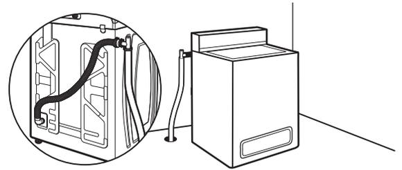
Floor drain system requires a Siphon Break Kit (Part Number 285834). Minimum siphon break: 28" (710 mm) from bottom of washer. Additional hoses may be needed.
