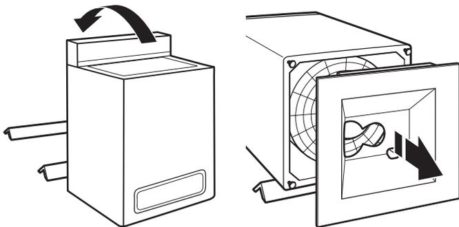
3. Remove tape from washer lid, open lid, and remove cardboard packing tray from tub. Be sure to remove all parts from tray.
