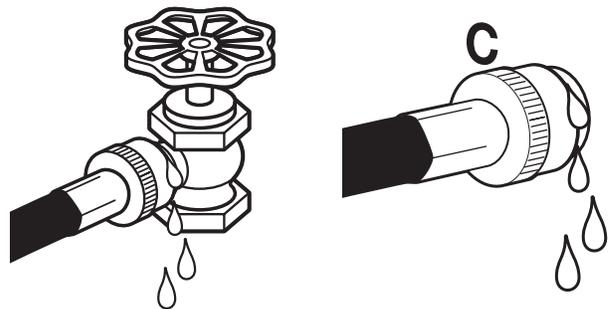
**NOTE:** Replace inlet hoses after 5 years of use to reduce the risk of hose failure. Record hose installation or replacement dates on the hoses for future reference.
