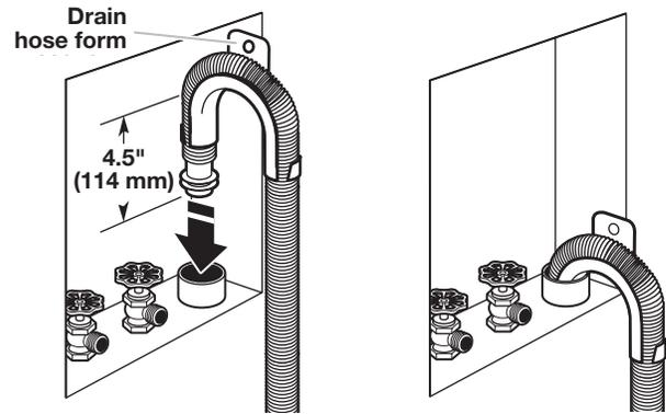
6. For floor drain installations, you will need to remove the drain hose form from the end of the drain hose. You may need additional parts with separate directions. See "Tools and Parts."
