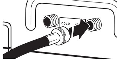
2. Attach hot water hose to hot water inlet valve marked with a red ring. Screw coupling by hand until it is snug.
