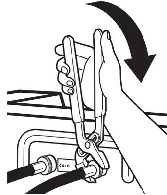
**NOTE:** Do not overtighten. Damage to the valve can result.
