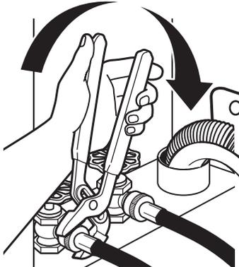
**IMPORTANT:** Do not overtighten or use tape or sealants on valve when attaching to faucets or washer. Damage can result.
