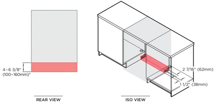
Service outlet at rear extends both sides, hoses and cords can be routed to either or both sides.
