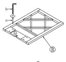
Place the top assembly upside down on a soft surface and pull out two wooden slides to each side. Install the cams on back panel to fix the leg frames. Note that on the cam there is an arrow showing the orientation of the cam to the pin. Adjust the cams in right
