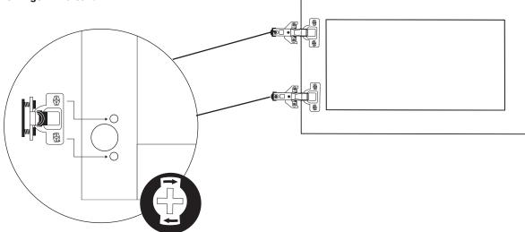
Note: The hinge can be separated by pulling the black tab and pulling apart the hinge from the hinge base. Separated hinges snap back together.
