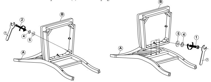
STEP 2: Attach the LSF/RSF Front Leg (C,D) to Wood Seat w/Seat Box (B) by using Flat Washer (5), Lock Washer (4) and Hex Nut (6) secure by Wrench (7). Attach Front Stretcher (E) and LSF/RSF Stretcher (F,G) to the LSF/RSF Front Legs (C, D) and Chair Back (A) by using Screw (3), tighten by a phillips-head screwdriver. Then insert Wood Glue (8) into the hole as picture shown. Fully tighten all bolts and screws at this time. Assembly product is now completed.
