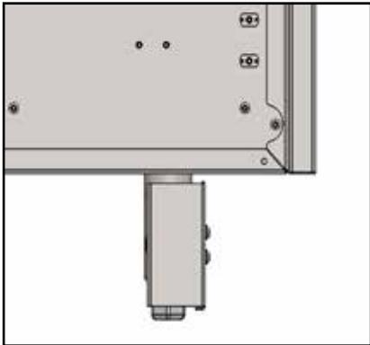
15. Side toe kicks connect in one of two ways, depending on the kitchen design. For island kitchens, the side toe kicks connect to the front and rear toe kicks. For kitchens against a wall, the side toe kicks connect to the front toe kick and the rear leg.
