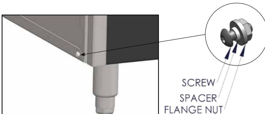
INSTALL THE SCREWS, SPACERS AND NUTS FOR MOUNTING THE END FINISHING PANELS
