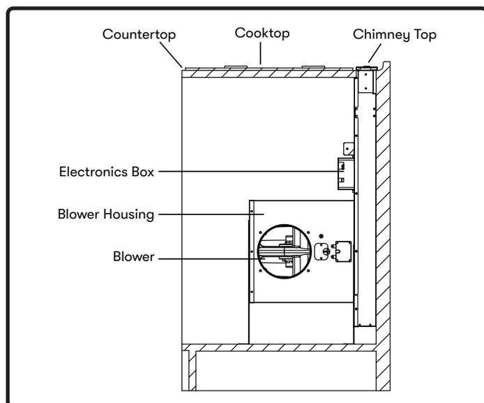
**NOTE:** The electronics box can be relocated to the left or right side of the blower housing.
