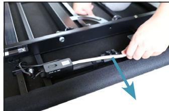
b. Disconnect The Wand to the control box cable via the 3-pin connector.
