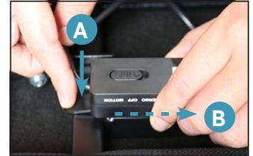
d. After removing the offline voice box, when installing on the other side, slide the wand device onto the mounting bracket until you feel it click into place.
