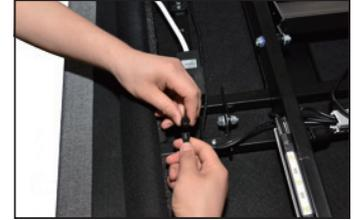
c. Press down the Mounting Bracket Tab (A); at the same time slide The Wand toward the USB ports (B) to remove the offline voice box.
