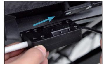
e. Connect The Wand to the Control Box Cable via the 3-pin connector.
