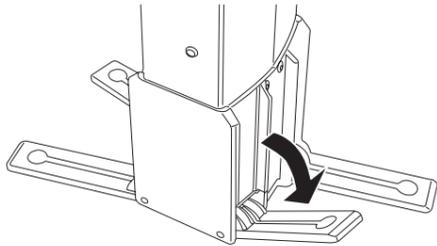
**CAUTION:** Make sure the feet are locked in place, or the screen could fall over.
